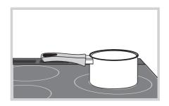
The areas marked with two concentric circles have an inner and an outer element. Turn the control knob clockwise to heat the whole area for larger pans - turn it the other way to just heat the inner part for smaller pans.
